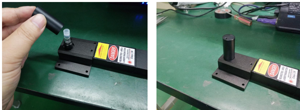
Fig. 9 Liquid sample measuring cell (liquid chromatography bottle, micro) (optional)
