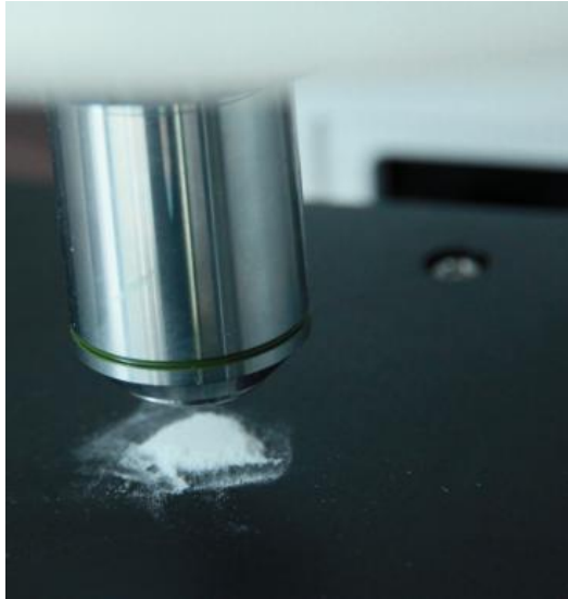
Figure 20 High transmittance objective for Raman signals. Objective focal length up to 8 mm.
