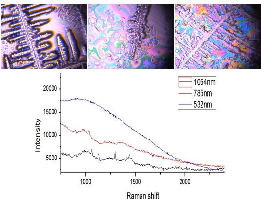
Fig 7 ATR8300TW experiment to measure cell metabolite, the above three picture surface topograph, the below Raman spectrum scanned by ATR8300TW-1064, ATR8300TW-785, ATR8300TW-532.
