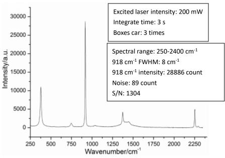
Fig 4 ATR8300TW acquire acetonitrile spectra
