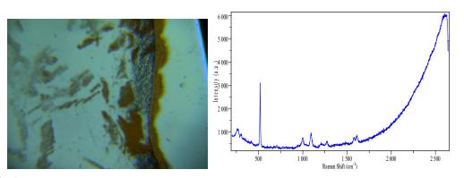
Fig 6 ATR8300TW SERS experiment (the Left is sample picture, the right shows SERS Raman spectra)
