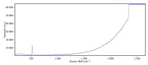
Fig 8 ATR8300TW measure Si Raman spectra (500mW, 1S integration time)
