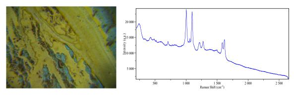
Fig 5 ATR8300TW SERS experiment 1 (the Left is sample picture, the right shows SERS Raman spectra)
