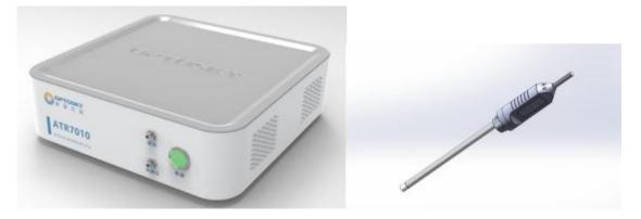
ATR7010 in-situ Raman Reaction Process Analyzer, the left side is the host, the right side is the probe(can be inserted into the reactor for measurement), and the middle is connected by an optical fiber(the length of the optical fiber can be customized, up to 100m)
