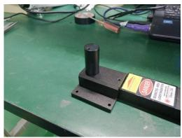
Figure 2 Liquid sample measuring cell (LC bottle, micro volume) (optional)
