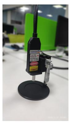
Figure 4 Fine adjustment stand (for solid and powder measurement)
