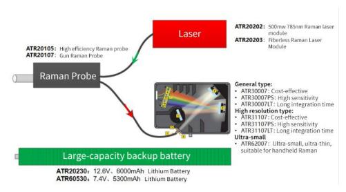
Figure 2 Raman spectrometer system composition structure
