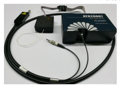
Figure 3 Raman system physical picture
